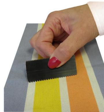
Equally spreading of adhesive
